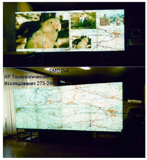
Small gap (~0.1 mm) technology for tiled screen of AR Technology
